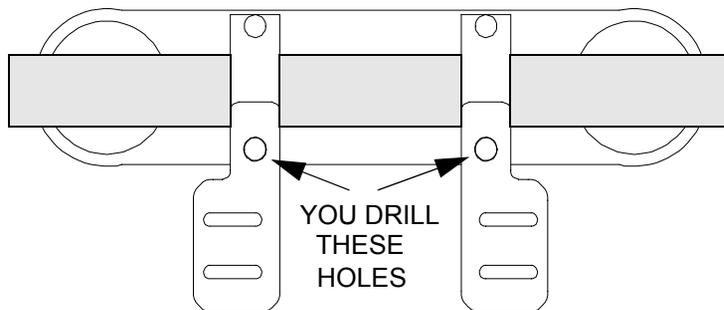
Use spacers between the bracket and clamp so that you have access to the bottom of the bracket for the nuts. Always drill the hole in the bracket tab as near as possible to the computer. Cut or grind off any unused portion of the bracket tab if necessary.
