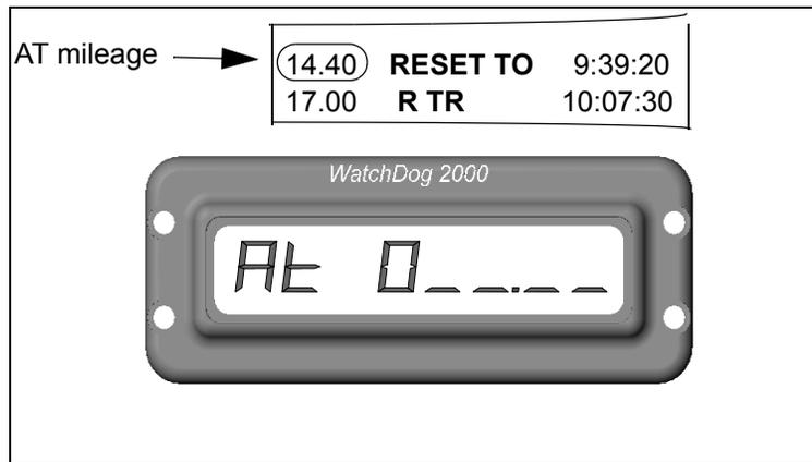
being edited. Use the **UP/DOWN** buttons to scroll through the numbers 0-9. Hit **MAIN** to select the currently displayed value for that digit field. The current digit will be accepted and the cursor will move to the next digit field. Continue entering the values for the remainder of the digit fields. When the last digit is entered, the display will change to “TO 0\_ \_ . \_ \_”, prompting you for the TO mileage of the reset. Enter
